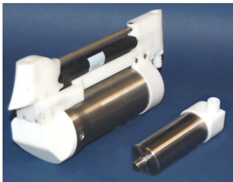
GPCTD with pump (shown with 1500 m titanium housing)
